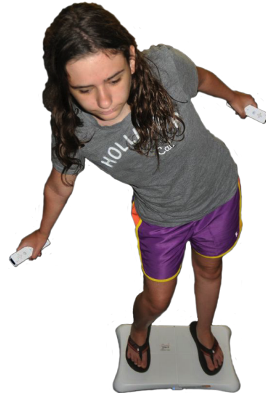
Figure 1: A child who is blind playing the nonvisual skiing exergame. Players control their speed by using their motion-sensing controllers as ski poles. A pressure sensitive input controller is used for input, where players lean to the left or to the right to pass through a virtual gate that is indicated using haptic cues.
