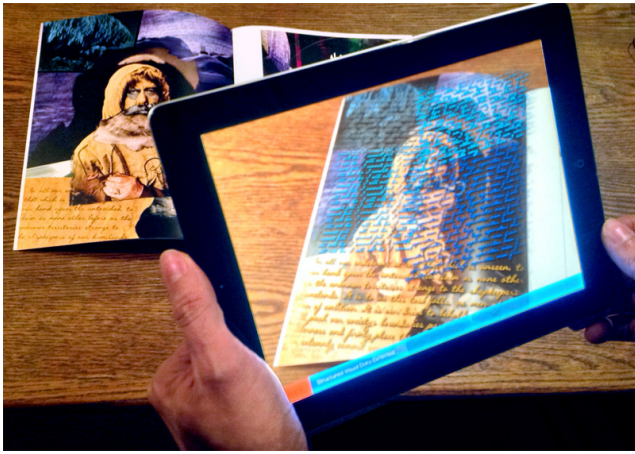
Figure 4: Interaction with the printed book using markerless tracking augmented reality.
