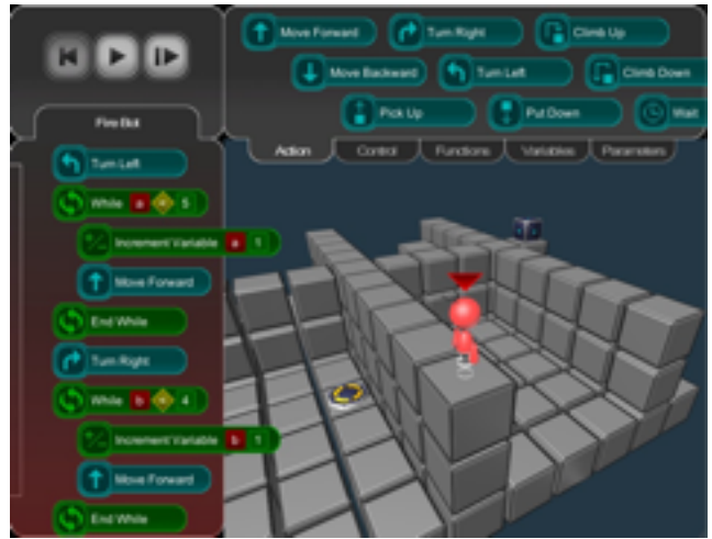
Figure 1: The BOTS interface. The robot's program is along the left side of the screen. The "toolbox" of available commands is along the top of the screen.
